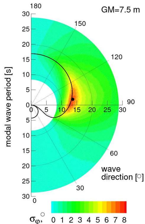
Figure 1: Calculated rms of roll angle for the loading condition with  $GM=7.5$  m at  $Fr=0.16$  in irregular waves vs. modal wave period and wave direction (radial and circumferential coordinates, respectively). Black line indicates resonance condition.
