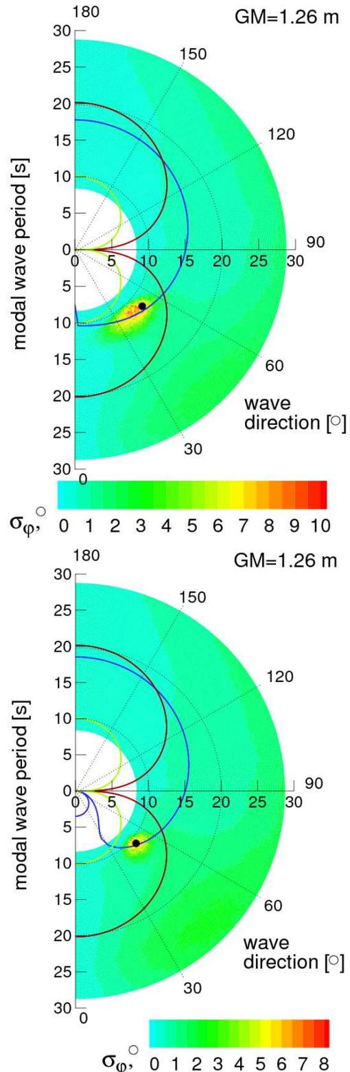
Figure 2: Calculated rms of roll angle for  $GM=1.2$  m at  $Fr=0.09$  (top) and  $0.12$  (bottom); the black points indicate representative scenarios for parametric resonance in quartering waves; blue line indicates resonance condition while yellow and green lines limit the area of suitable wave lengths.
