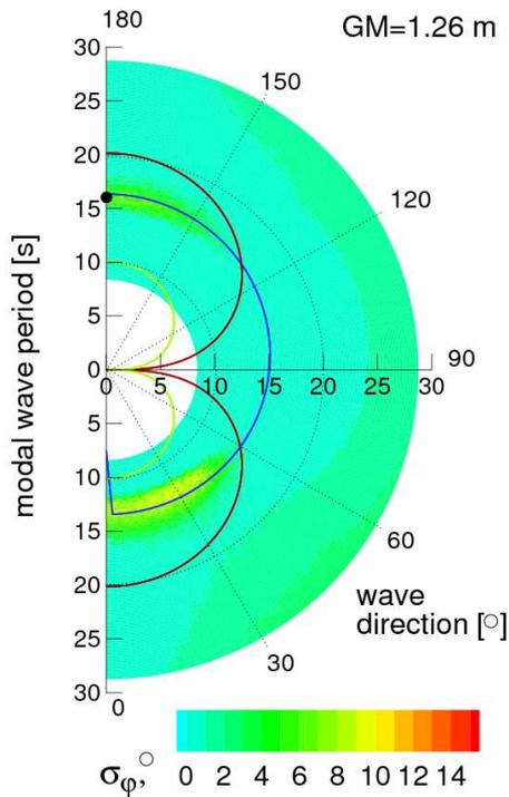
Figure 3: Calculated rms of roll angle for  $GM$  of 1.2 m and  $Fr$  of 0.04 in irregular waves. Black point indicates selected case for parametric resonance in bow waves; blue line indicates resonance condition, yellow and green lines limit the area of suitable wave lengths.
