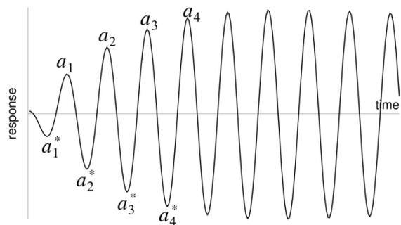
Figure 5: Post-processing of responses in regular waves.
