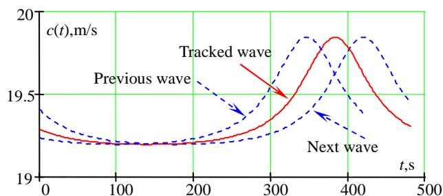
Figure 5: Celerity of the two-component wave tracked in Figure 4, along with the celerities of the previous and next waves
