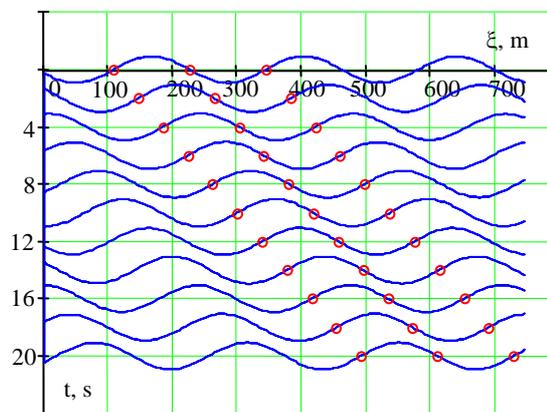
Figure 4: Zero-crossing points of two-component wave
