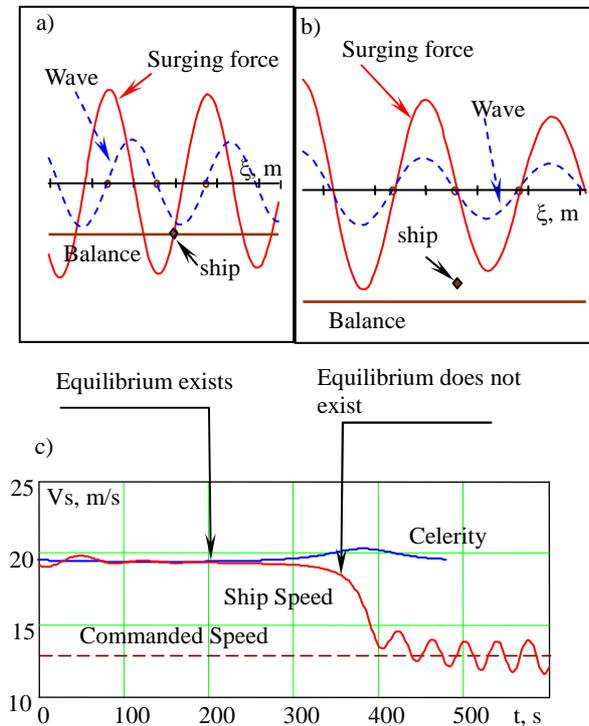
Figure 6: Release from surf-riding in two-component waves:
