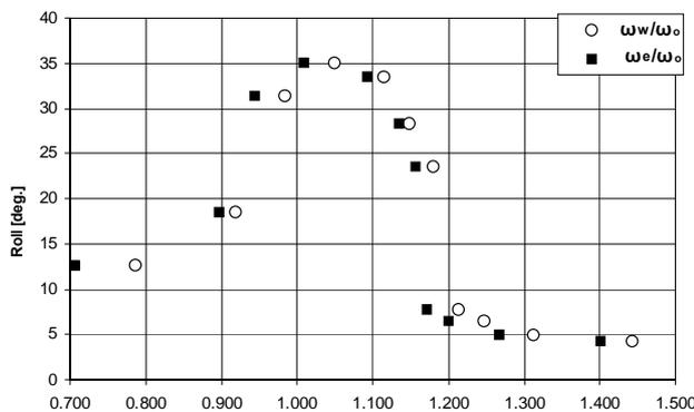
Figure 11: Roll response diagram for  $H/\lambda = 1/30$ .
