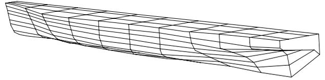
Figure 6: Half-hull panelization.
