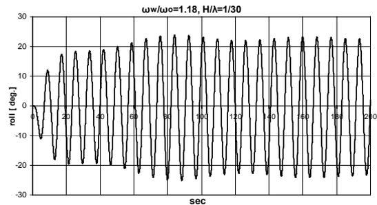
Figure 8: Roll response in beam waves
