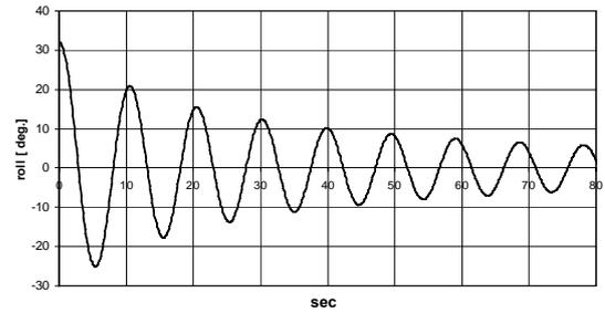
Figure 7: Roll decay test
