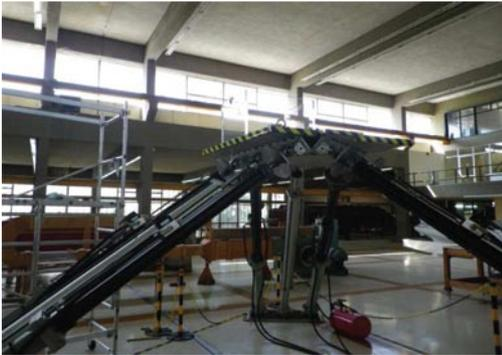
Figure 1. The shaking-table of the School of Naval Architecture and Marine Engineering, National Technical University of Athens.
