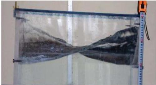
Figure 3. Combined wave in longitudinal and in transverse direction. The tank is excited along the gravity vector. The tank presents a slight tilt around the transverse axis.
