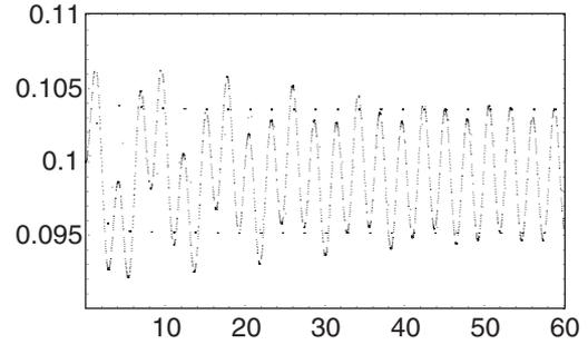
Figure 1. Comparison of responses (continuous line corresponds to 3rd order model):  $U = 5$  m/s,  $k_1 = 3$ ,  $k_2 = 1$ ,  $\psi_0 = 0.1$  rad,  $\psi_r = 0.1$  rad.
