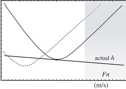
Figure 6. The condition of parametric yawing is produced by the intersection of the curves of actual and critical  $h$ . The position of these curves depends on proportional gain; however that of  $h_{cr}$  is very sensitive to the differential.
