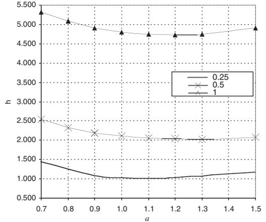
Figure 7. Numerical boundary of parametric yawing for large  $\zeta$ . By  $a$  is meant the ratio  $4\omega_0^2/\omega_c^2$ .
